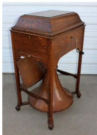
Figure 6: Schoolhouse Victor XXV with hidden horn
